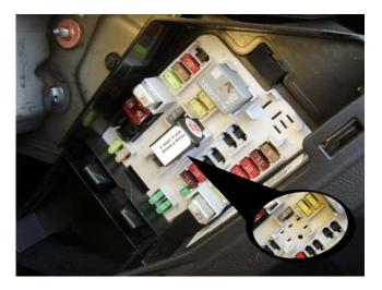
Test by pressing trunk release on the fob (or release button in interior) twice, to open the trunk. Replace panel after verifying operation. That's all there is to it! *Note that the Two-Shot relay indefinitely remembers the first press and will release the trunk on the second press of the button.*
