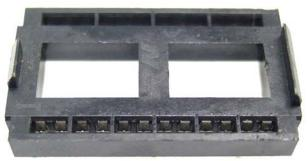
This socket was produced with a standard 0.6" lead spacing and was designed to accommodate the standard chip carrier commonly used on all of the turbo cars. Here is a bottom view of this socket:
