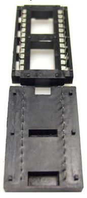
Note the comparison of the pin spacing between the late design (foreground) and the early design. The socket had a closed bottom and the pins were 12 mm apart as opposed to .6" as found on the earlier RN socket. The receiving ends (top) of the sockets, however, are similar in design so that they both can accept the standard RN carrier. Since the difference in lead spacing is minimal, the replacement socket, early style, can be used to replace the socket on all years of ECM's.
