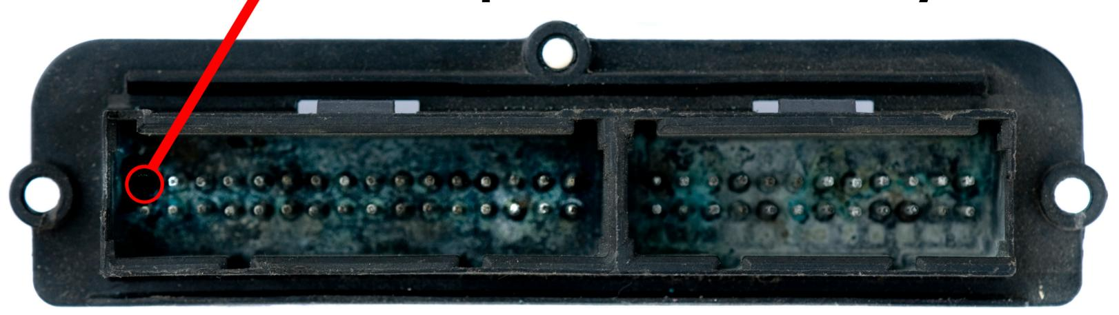
Green and white corrosion due to presence of water in the connector.
