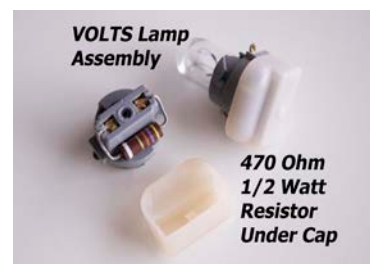
Left: Resistor Bulb Socket. Right: inside view of the specially made socket with a 470 ohm resistor.
