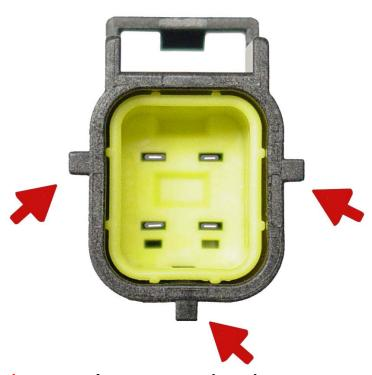
Keying tabs (red arrows) may need to be removed from existing connectors to facilitate installation
