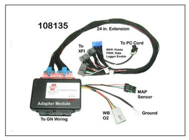
Pink wire is <u>Data Logger Enable</u> connection. White wire is <u>Points</u> signal for MSD add-on.
