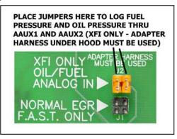
The jumpers are installed at the factory in their "NORMAL EGR" position as shown in the image on the left. To use the pressure logging function, you will need to remove the jumpers and relocate them as shown in the image on the right. Additionally, there is an internal relay on the PC board that interfaces with the external fuel pump relay. This relay provides the correct interface between the ECU and your factory fuel pump relay.
