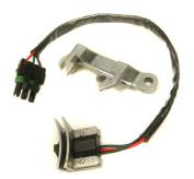
Your original 1984-1985 crank sensor looks like this. It is obsolete and no longer available from GM. Note the wider sensor opening on the bracket and slot on one end.
