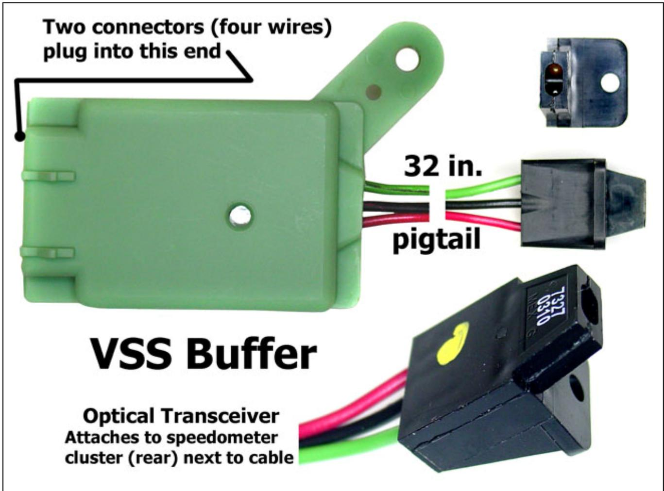
The VSS Buffer Module is designed to intercept a signal from the movement of the speedometer cable, and transmit a filtered signal to the ECM and to the Cruise Control Module. This signal is relative to the speed of the vehicle.
