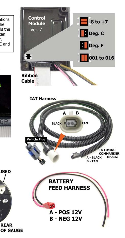
There are two connectors on the controller module; one red and one black. The red connector attaches to the extension which has two wires; black and pink/black stripe. The striped pink wire (cavity A) must be attached to a switched 12 volt source, typically an accessory feed. Use a voltmeter to determine the switched voltage source, which turns off when the keyswitch is off. The black wire (cavity B) goes to battery negative and must be grounded to the vehicle frame.
