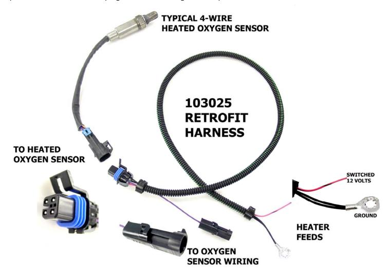
Attach the pink/black stripe wire to any device under the hood that produces **SWITCHED 12 volts** from the battery. The heater in the sensor uses about 1-1/2 amps of current. Be sure the supply wire from the engine harness can handle the additional current load.
