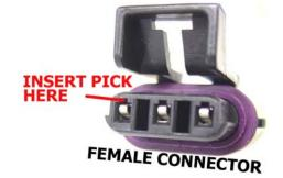
Using the pick, insert into the connector as shown, then pull the wire with the terminal out of the rear of the connector body.
