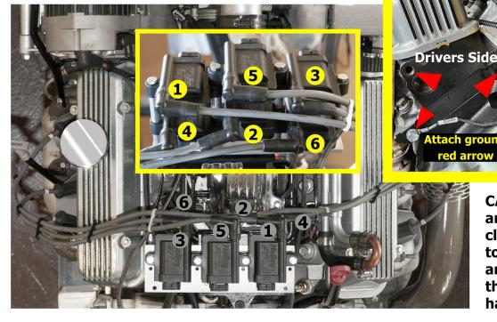
CAUTION: Be sure to anchor the coil harness close to the coils as shown to prevent the windshield arm link from contacting the coil connection harness.
