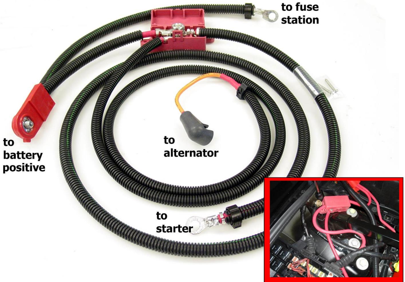
This harness uses a high temperature convoluted conduit for the section that runs down to the starter stud. This is necessary because of the limited clearance when running upgraded headers.
